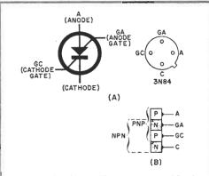
Fig. 1. Lead identification of the SCS including bottom view of the base. Unlike its SCR cousin, the SCS has an anode gate.
