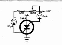
Fig. 3. In (A) above, the pnp section is inoperative. In (B) below, npn section is inoperative. In both circuits, set the pot to full maximum before turning on the power.
