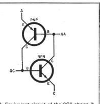
Fig. 2. Equivalent circuit of the SCS shows it to appear to be two conventional bipolar transistors tied in a regenerative-type circuit.
