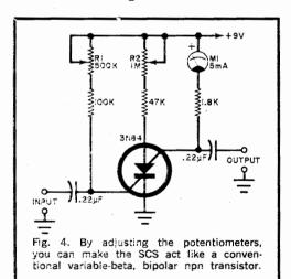
With potentiometer R2 set at maximum resistance, the circuit operates as an npn transistor amplifier. With R2 set on minimum resistance, the circuit is simply a turned-on SCS. In between these extremes, the circuit is regenerative, with its gain increasing as the value of R2 is made smaller.
