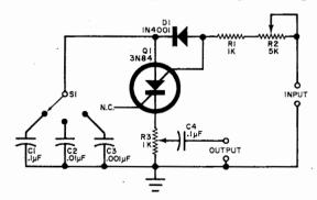
This simple self-powered pulse generator can be built directly into an existing audio sinewave generator. The output pulses can be used to trigger experimental digital circuits or, if accurately calibrated, scope trace times.
