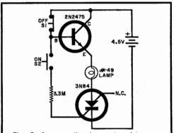
Fig. 6. A conventional npn transistor can be used in place of a power switch to turn the SCS on and off. Any type of mechanical contacts can be used for switches S1 and S2.
